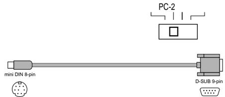
If you use an 8-pin MINI DIN to 25-pin D-SUB cable, connect a 25-pin to 9-pin plug adaptor to the D-SUB end of the cable.
